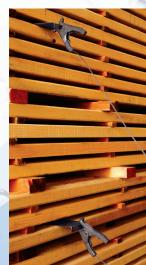
Heavy Duty Clamps At tached to Sensors
