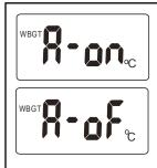
Press **MODE** to select HI WB (WBGT) alarm ON/OFF.
