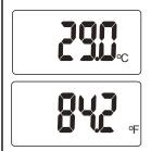
Press **POWER** button to save WBGT setting, and meter will go back to normal measurement.
