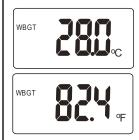
When WBGT alarm is on, HI WB (WBGT) icon with the current alarm threshold appears on the LCD. Press **MODE** button to increase the alarm threshold from decimal point (0.1-0.9), to unit digit (0-9), then ten digit (60-90°F/20-30°C) until you release the button.
