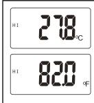
When HI alarm is on, HI icon with the current alarm threshold appears on the LCD.
