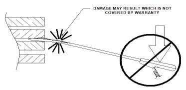
DO NOT APPLY VERTICAL PRESSURE TO HANDLE WHILE PROBE TIP IS STILL IN STACK.
