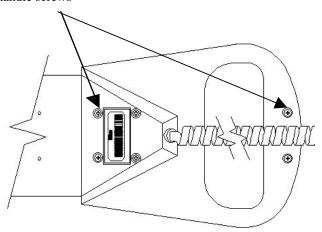
• **Step 2.** Disconnect the old cord from the coupler. Depress lever and extract plug from coupler.
