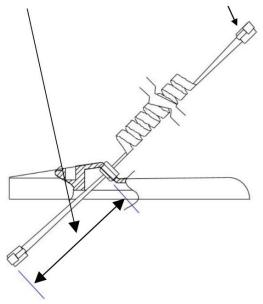
• Step 5. Connect replacement cord to coupler. Ensure latch clicks into detent.
