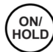
When the meter is in the inspection mode, and the On/ Hold button is momentarily pressed and released, it will enter Hold mode to allow the user to “freeze” the moisture reading.
