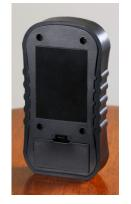
function buttons as well as the display screen, sensing plate, and battery compartment are accessible without removal of this rubber guard. The boot will fit on the meter only one way correctly. Failure to correctly place the boot will result in inaccurate readings.
