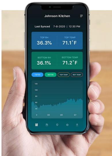
**It's your constant guardian.** When installed, the Floor Sentry will give you around 8 years of constant temperature and RH monitoring. Using the free Wagner Sentry® app, you can check your floor conditions at any time. You can also set alarm thresholds to capture spikes in temperature and RH in your floor and alert you to these potentially damaging conditions when you are in Bluetooth® range of the embedded Floor Sentry.
