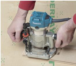
3) Use a router or similar device to create a space for the Floor Sentry in the underside of the wood floor plank.
