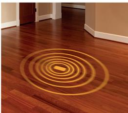
6) At any time, for days, months, or years after the installation, you can open the Wagner Sentry app and connect with your embedded Floor Sentry devices. Once connected, you can set the time intervals in which the Floor Sentry will record and store RH and temperature readings, configure readings alarm thresholds to trigger push notifications, and more.
