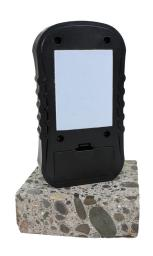
This protective boot should remain in place at all times even when calibrating your meter with the On-Demand Calibrator.\* All function buttons as well as the display screen, sensing plate, and battery compartment are accessible without removal of this rubber guard. The boot will fit on the meter only one way correctly. Failure to correctly place the boot will result in inaccurate readings.
