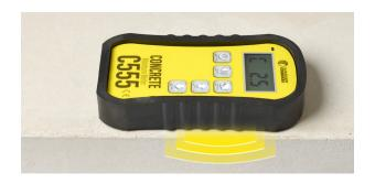
4. Be sure to press down with slight but firm pressure to ensure good sensor plate contact with the surface of the concrete.
