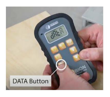
10. Press the DATA button, followed by UP or DOWN, to make sure the meter displays Data "ON" (for manual mode), or "AUTO" (for automatic data collection mode). When done, press DATA again to confirm and then ON/HOLD to return to Standard Measurement Mode.
