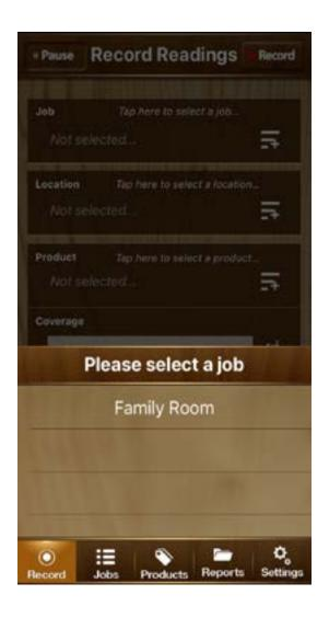
4. Press "Record," then press "Job" at the top of the page to select the appropriate job name. If necessary, press (+) to select another job, location, or product. The pen icon can be used to change a product description, i.e., "Spindle" or "Leg."
