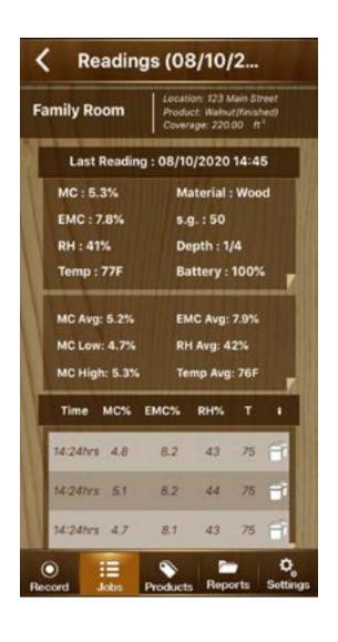
15. Press the right-facing arrow next to the date to see the statistics of the selected job on the Readings screen. The product is listed in the upper right box to distinguish if working with multiple products in the same job. This is also the screen where individual readings can be deleted if necessary. Just click the trash icon next to the reading and select "OK" to delete.
