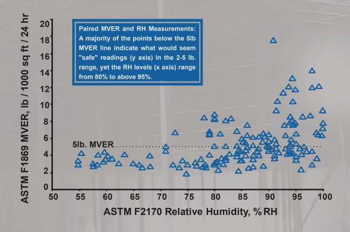
"There are many reasons why calcium chloride moisture emission testing cannot do what a relative humidity test can accomplish. The bottom line is that RH testing is a far better predictor of whether or not a floor covering or coating on a concrete slab will succeed or fail. It is unnecessary to perform moisture emission tests in addition to relative humidity."
