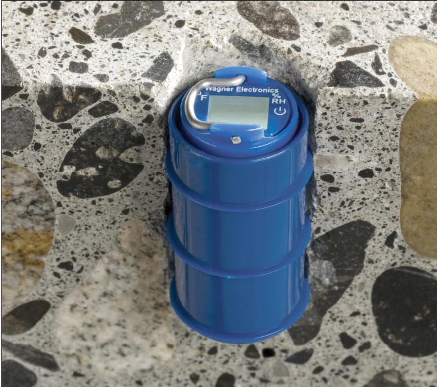
Modern electronic thumb-size relative humidity probes now are available that can be placed below the surface of the concrete slab to monitor drying without interfering with construction or use of the floor. The devices provide real-time relative humidity and temperature at the push of a button. Photo: Howard Kanare
