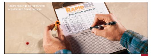
If using the Smart Reader with the DataMaster<sup>™</sup> app, the in-hole ambient relative humidity and temperature readings will appear on the screen of your Apple or Android device within approximately two seconds. Immediately remove the Smart Reader.
