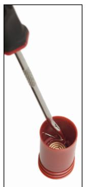
the tool counterclockwise while pulling up. If you are going to be doing future testing of this hole, make sure you put a protective cap on the sleeve. When ready to obtain additional readings, you can just reverse the above removal process to reinstall the Smart Sensor into the Base Sleeve.
